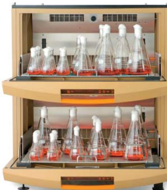
\*A 3mm orbit (or throw) with maximum 1000 rpm is available for growing in microtiter plates.
