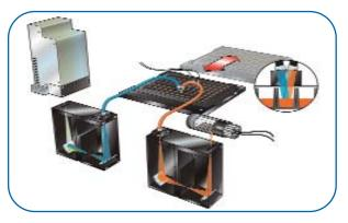
The Synergy 4 monochromator system uses two double-grating monochromators. Highest stray light rejection, continuous wavelength selection, spectral scanning: this system combines high performance with convenience and flexibility.
