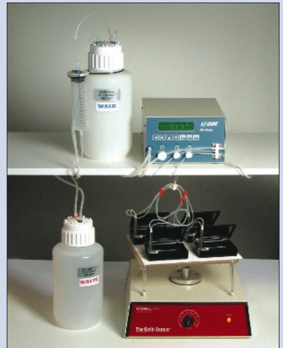
LI-COR Blot Washer configured for washing and secondary antibody incubation of four blots in incubation boxes. Shown with optional shaker (The Belly Dancer®, Stovall Life Science Inc.).
