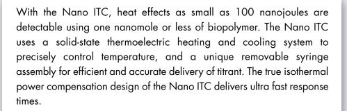
The TA Instruments Nano ITC is engineered specifically for binding and kinetics studies on purified dilute biological samples of limited availability
